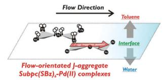
Two-phase Couette flow linear dichroism measurement of the shear-forced orientation of a palladium(II)-induced aggregate of thioether-derivatised subphthalocyanines at the toluene/glycerol interface
